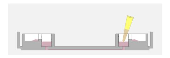
**Important**: Note that the channels should never dry up. Take incubation times into account and use the evaporation reservoirs as long as possible.
