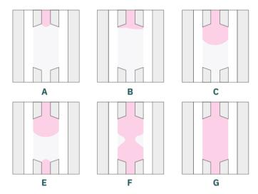
b. **Inject the solution (10 μL) slowly** into the chip. First, the meniscus will enter into the chamber (A). Continue until the chamber is fully filled (B-F).
