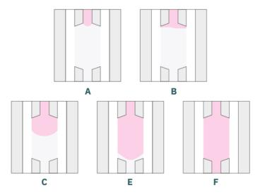
**3. Flip the chip upwards and downwards** every 30 seconds for a few minutes for **homogeneous 3D distribution** during the polymerization of the hydrogel.
