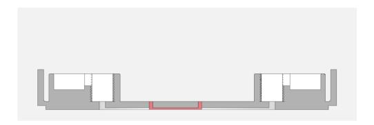
**4.** Seal the central chamber inlet and outlet with the adhesive provided. Make sure that the surface is clean to ensure proper adhesion.
