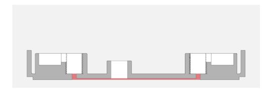
**Tip:** When seeding a monolayer underneath the membrane, flip the chip downwards and incubate for better coating deposition on the membrane. In this case the volume must be the one that fits in the channel.
