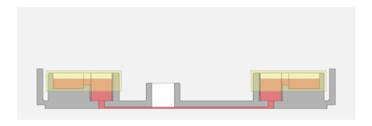
**Remember:** Beonchip membranes are not impermeable, they are porous. During 2D culture, if the monolayer underneath the membrane is not completely confluent, medium may go through the membrane.
