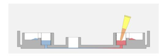
**Tip**: You may **tilt the device** manually in order to ease the dilution buffer **flow several times** from one reservoir to another before you remove it.
