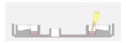
**Important**: Note that the channel should never dry up. Take incubation times into account and use the evaporation reservoirs as long as possible.
