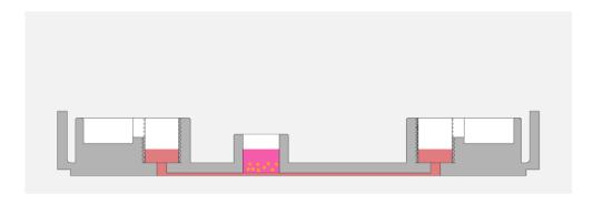
Make sure that all the medium **has been depleted** from the reservoirs and inlet/outlet to avoid spilling medium when flipping the device.
